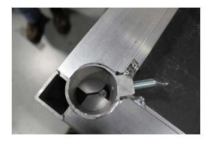
2. Remove deck screws from edge of aluminum frame, down the length of the center brace and in the corners.
