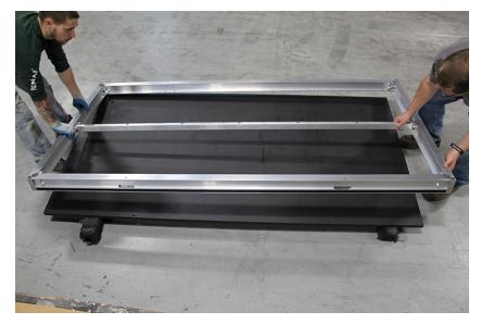
4. Place frame over new surface & use rubber mallet to bang frame securely in place on new surface.
