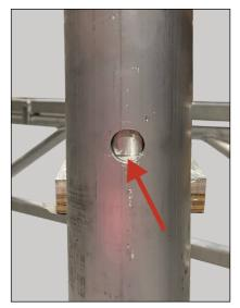
10. Insert plastic stripping into hole & feed while turning leg until completely inside outer locking hole:
