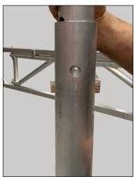
11. Slide inner leg up & down to make sure it's working / remove wood:
