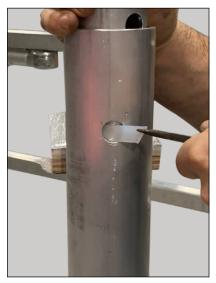
7. Rotate inner leg while pulling on stripping & remove strip:
