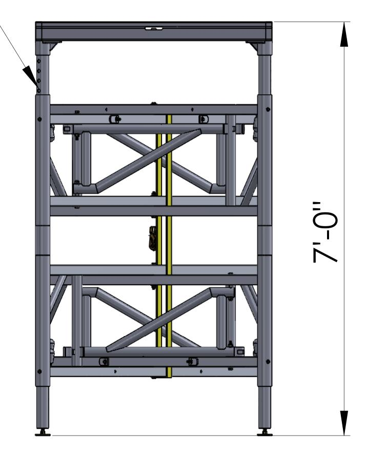
RATCHET STRAPS MUST BE INSTALLED STRAPPING THE TOP AND BOTTOM HORIZONTAL MEMBERS OF THE WUNDERSTRUCTURE TOGETHER
